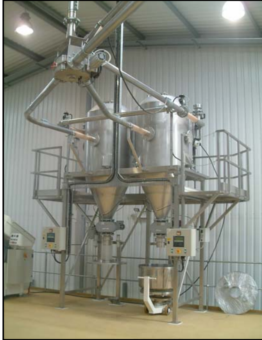
Picture above: Ingredient dispensing hoppers each with a capacity of 350kg.
