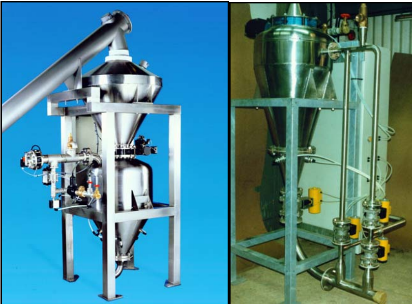
Picture above and below: Dense phase conveying pots designed and supplied by STB for various powder conveying systems.
