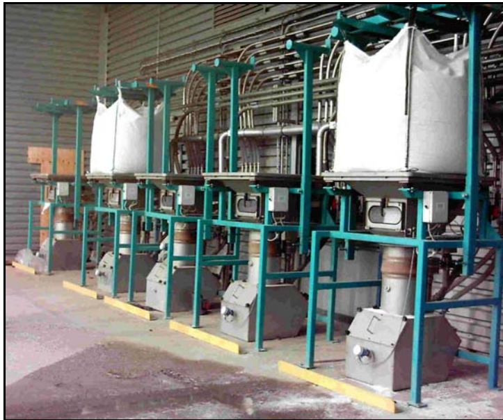
Picture above and below: Line of big bag dischargers transferring various ingredients into a STB pneumatic conveying transfer system. Dischargers are manufactured in painted mild steel or stainless steel. Bags can be loaded on to stations by fork truck or by lifting hoist. STB offer a choice of transfer conveyors: mechanical screw conveyors, vibratory feeders or pneumatic conveyors
