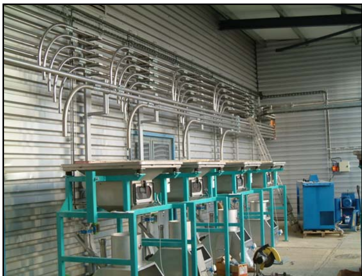
Picture above and below: Line of big bag dischargers transferring various ingredients into a STB pneumatic conveying transfer system. Dischargers are manufactured in painted mild steel or stainless steel. Bags can be loaded on to stations by fork truck or by lifting hoist. STB offer a choice of transfer conveyors: mechanical screw conveyors, vibratory feeders or pneumatic conveyors
